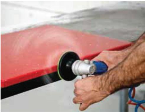
■ Polishing any Çimstone edge profile should be done in a progressive manner using only granite or marble diamond polishing pads.
